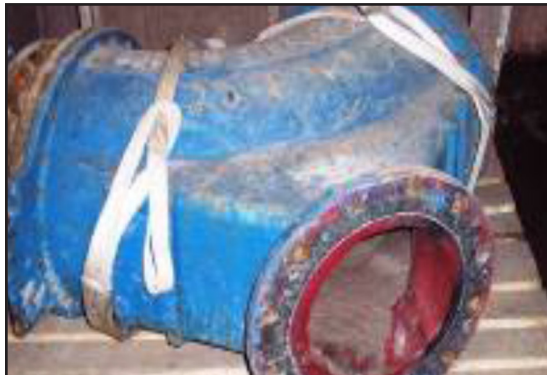
Rubber-lined valve body suffering from rubber delamination
