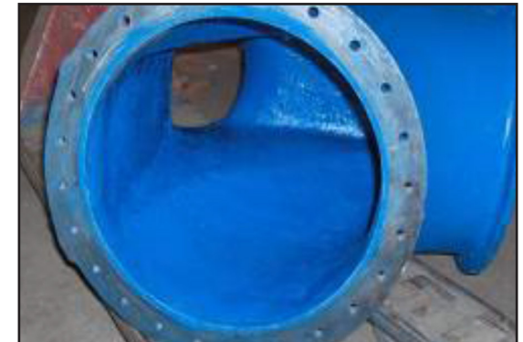
Completed valve body ready for service
